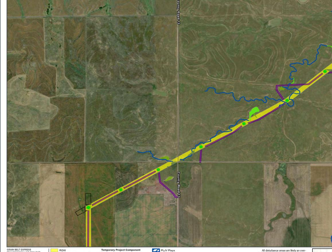
Permanent Project Component Transmission Structure Habitat Conversion Vegetation Clearing Temporary Project Component Access Road Pull Site/Tension Site Hydrology Delineated Stream
