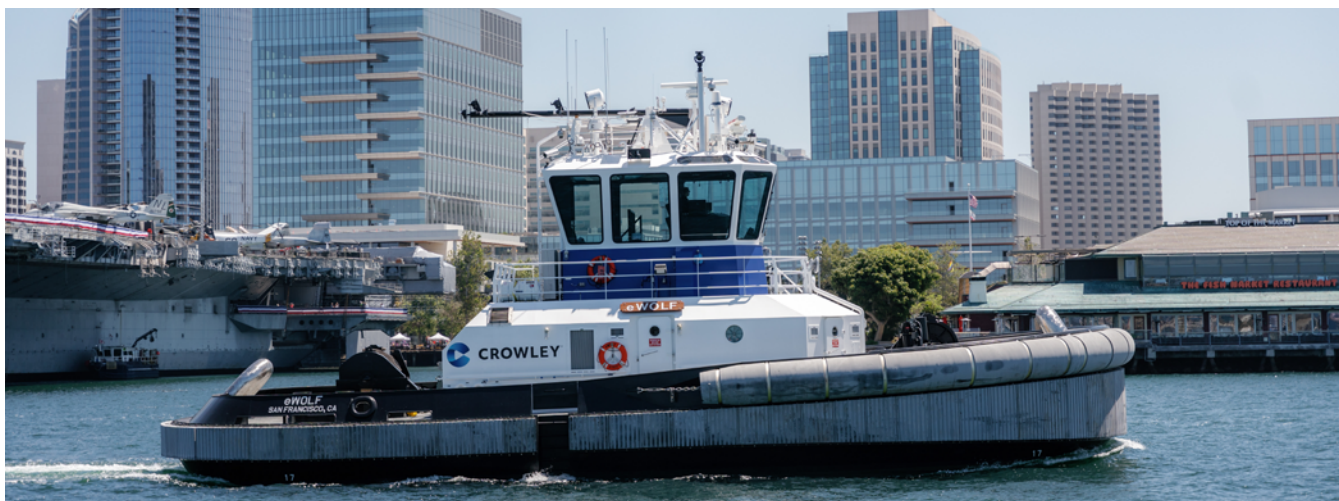
The Crowley e-Wolf, an electric tug, operating in the Port of San Diego. Image courtesy of Crowley.
