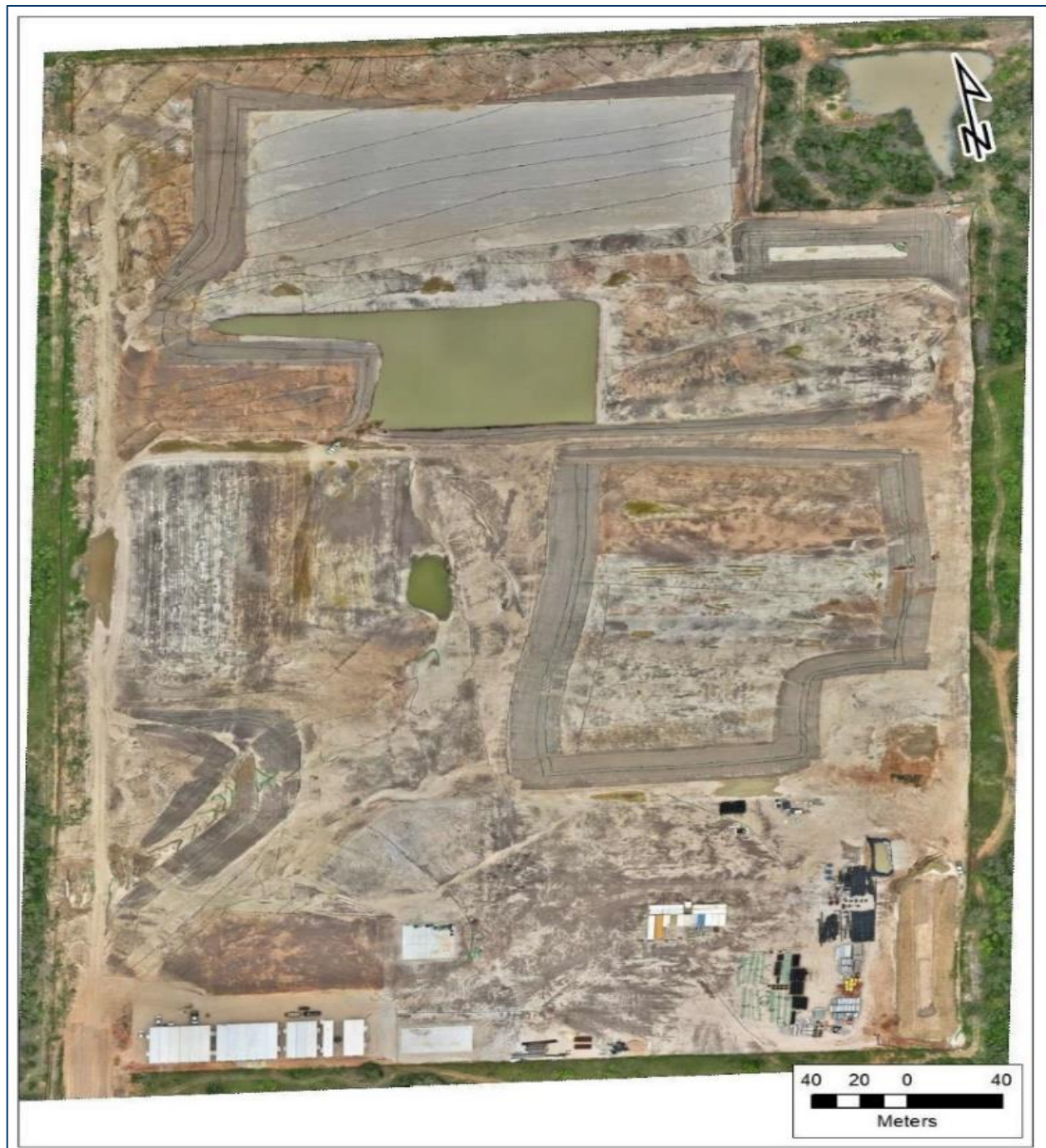
Figure 3a: Existing Conditions, May 2024, Project Site Main Facility – Cleared and Graded with Construction Staging Area and Temporary Stormwater Detention
