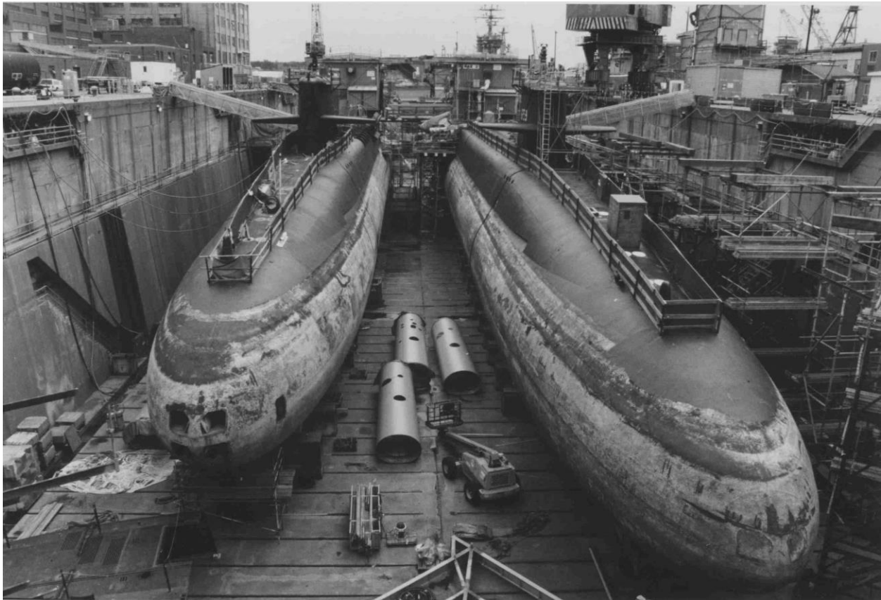
Submarines in Drydock for Defueling, Reactor Compartment Removal, and Recycling
