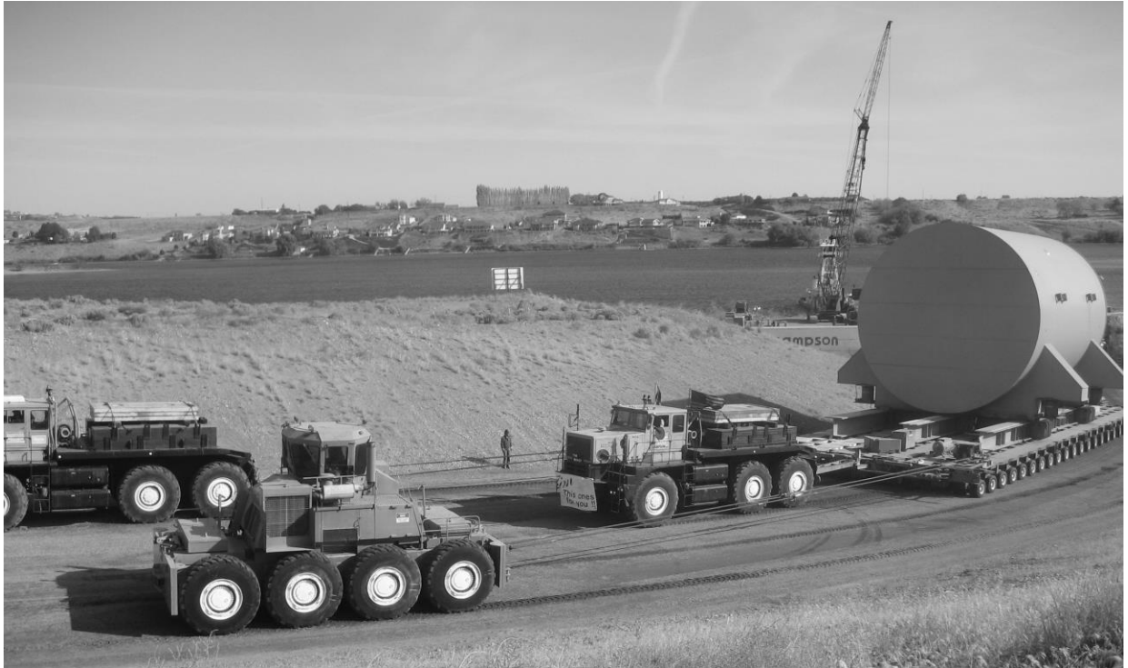
Reactor Compartment Package enroute to the Disposal Trench
