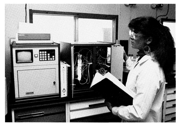
Checking a Total Organic Carbon Analyzer Run
