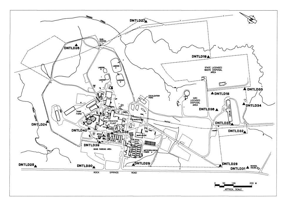
Figure 2-9. On-Site Thermoluminescent Dosimetry (TLD) Locations.
