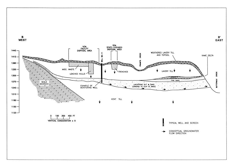
Figure 3-2. Geological Cross Section Through the South Plateau.
