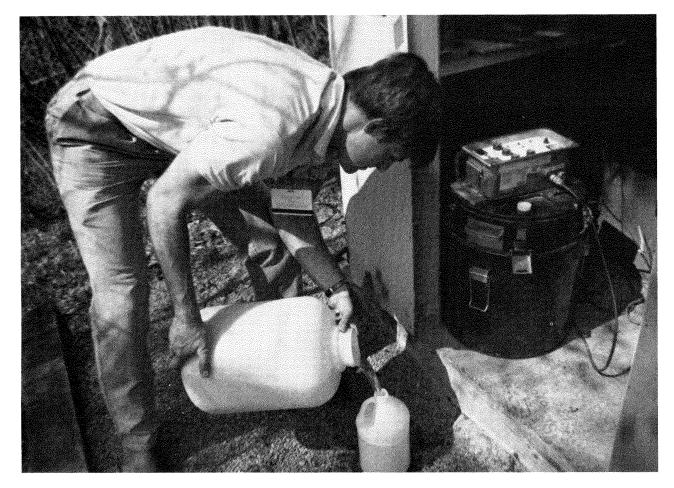
Collecting a Sample at a Continuous-Stream Sample Station
