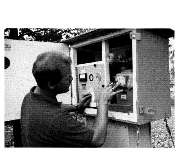
Recording Air Flow at an Environmental Air Sampler
