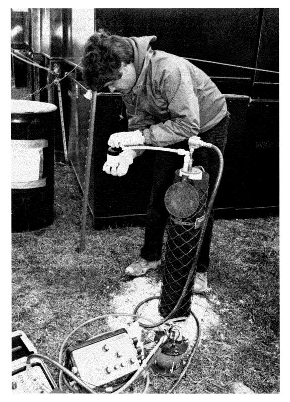
Sampling with a Dedicated Bladder Pump Installed in an On-site Groundwater Monitoring Well
