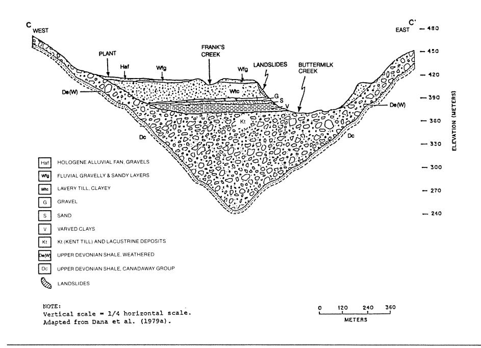
**Figure 3-1.** Geological Cross Section Through the North Plateau.
