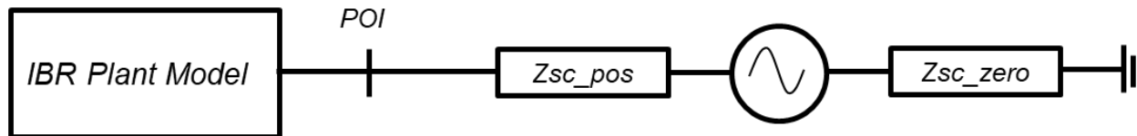
Single Machine Infinite Bus Test Case
