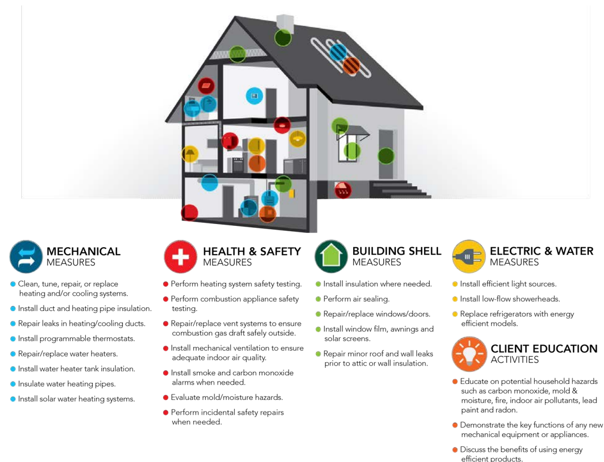
Figure 3 | Typical Weatherization Measures
