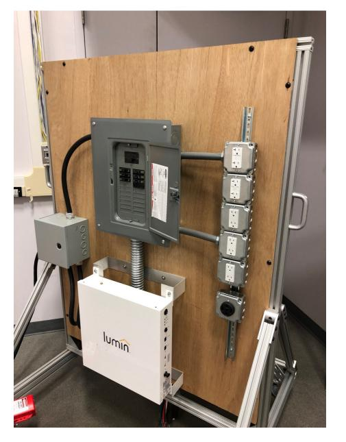
This test rig allows evaluation of power sharing technologies, such as smart panels, subpanels, smart breakers, and responsive end-use devices.
