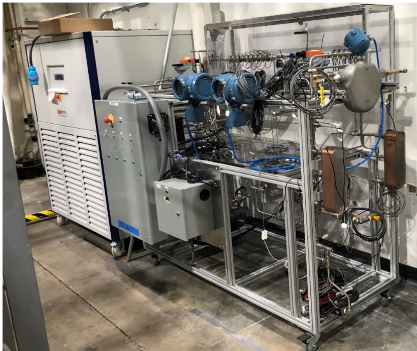
Liquid-to-refrigerant heat exchanger test rig
