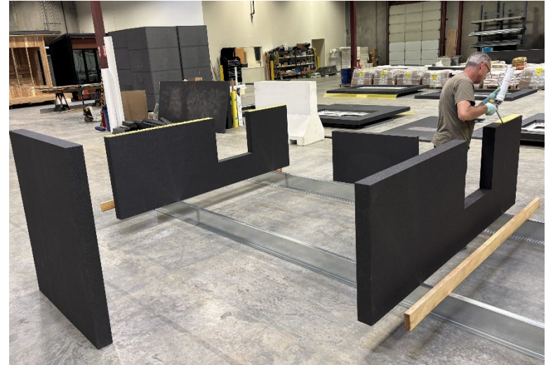
Wall panel fabrication in factory during Stage A retrofit; window frame and door cutouts prepared for window frame attachment.
