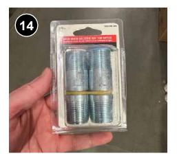
If not provided by the manufacturer, install heat traps on the inlet and outlet piping. 7.0302.3k.
