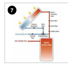
Install the storage tank in compliance with applicable code and manufacturer specifications. If conflict exists between code and manufacturer specifications, apply the more restrictive requirement (e.g., seismic straps may be required in some areas). 7.0302.6d.
