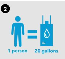
Installations must be sized according to "*Residential Solar System Sizing Verification*," which uses a 20 gal/ person standard.
