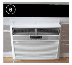
Ensure the supplied electrical cord is of sufficient length to reach the nearest outlet that meets the requirements of **NFPA 70 Article 422** (Maximum breaker size for the circuit matches the breaker marking on the appliance). If the cord does not reach, proceed with one of the following options, based on the recommendation of the auditor and available funds:
