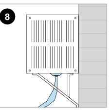
Attach the drain hose (if supplied) to the outside of the air conditioner. Ensure condensate drains away from the building and any other items that may be damaged.
