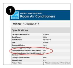
Double check the name plate of the new unit to ensure the new unit meets the requirements of the program. The new unit must match existing voltage and have a CEER of 12 or higher of the same or lesser capacity (when compared to the unit it is replacing). 5.0301.1b.
