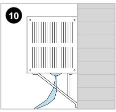
Attach the drain hose (if supplied) to the outside of the air conditioner. Ensure condensate drains away from the building and any other items that may be damaged.
