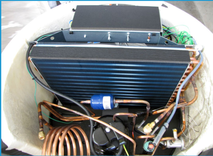
Figure 2. Photos show the inside of a heat pump, taken during the set-up of a heat pump water heater experiment at the National Renewable Energy Laboratory. Heat pump water heater technology has the potential to save twice as much energy when compared to an all-electric water heater because it utilizes the heat in the surrounding air instead of relying solely on electric resistance to heat the water. Photos by Kate Hudon, NREL 19461 (left) and NREL 19462 (right).
