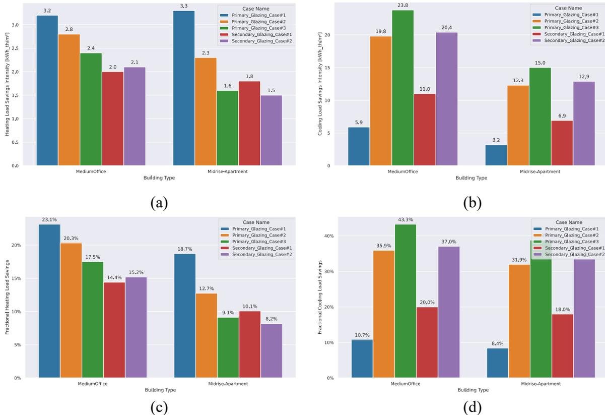
**Figure A-11. Benefits of proposed window measures, including (a) annual heating load intensity savings, (b) annual cooling load intensity savings, (c) fractional heating load savings, and (d) fractional cooling load savings.**
