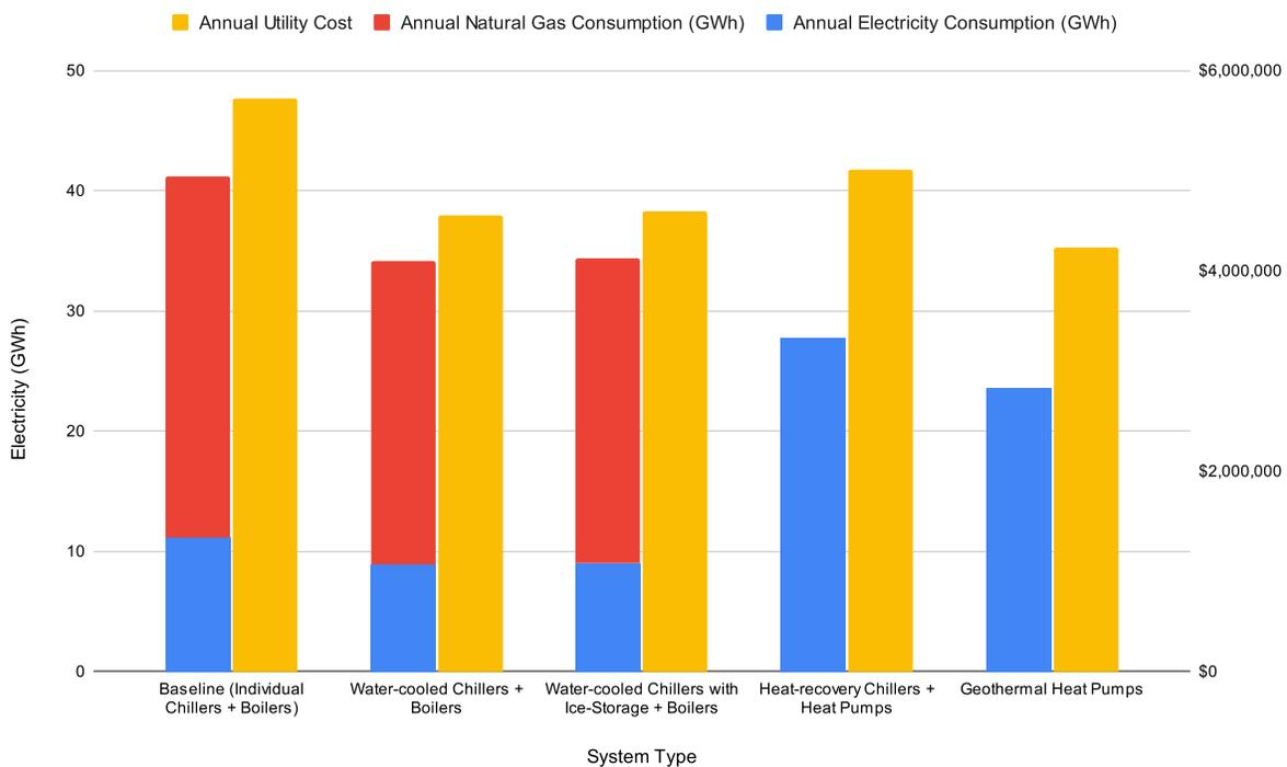
**Figure A-12. Annual energy consumption and cost comparison between baseline and proposed DES system configurations.**
