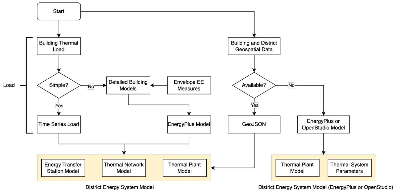
**Figure A-9. Schematic diagram of the proposed DES modeling framework.**
