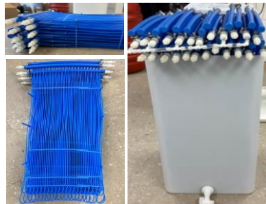
ORNL-developed PCM heat exchanger and low-cost salt hydrate PCM
