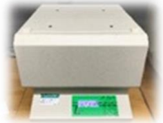
ASTM Heat Flow Meter
