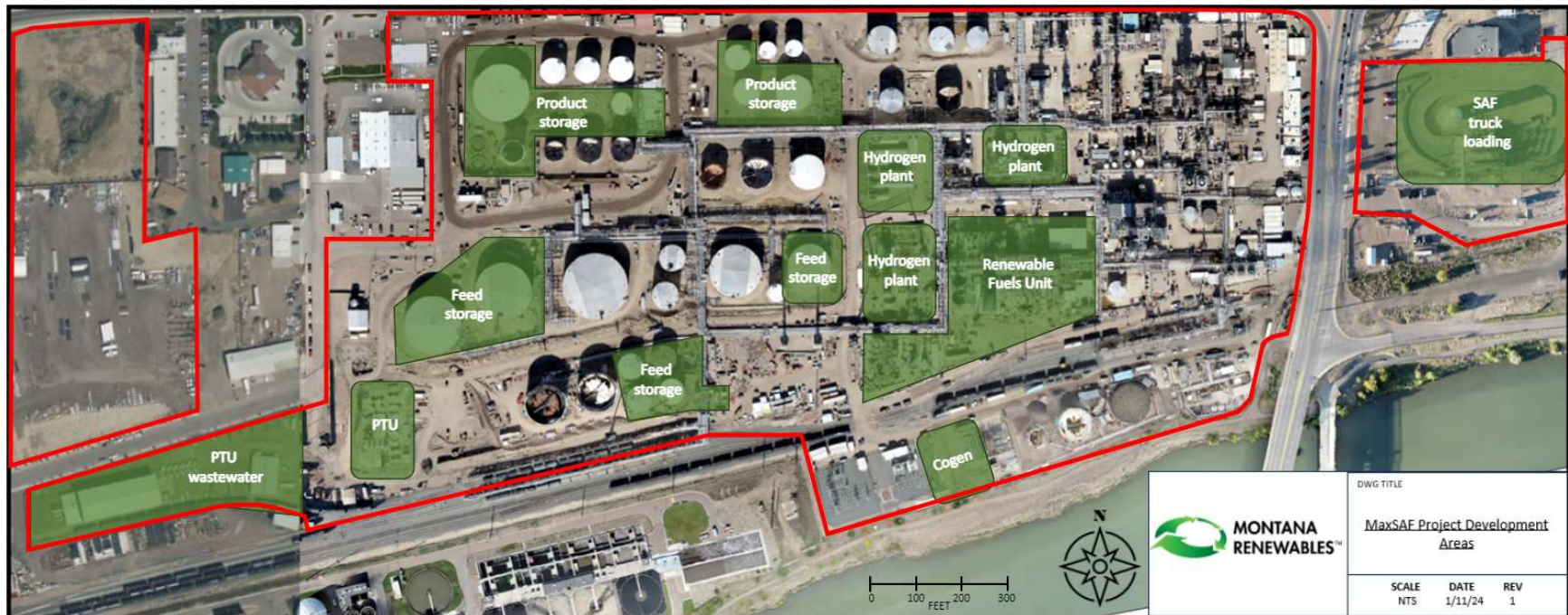
Figure 2. Renewable Fuels and Biomass Facility Conceptual Layout
