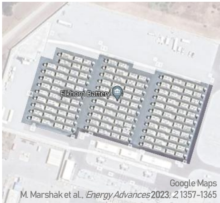
Elkhorn Battery in Moss Landing, CA (Tesla Megapack 2 XL) 730 MWh, 13,500 m 2 , 54 kWh/m 2
