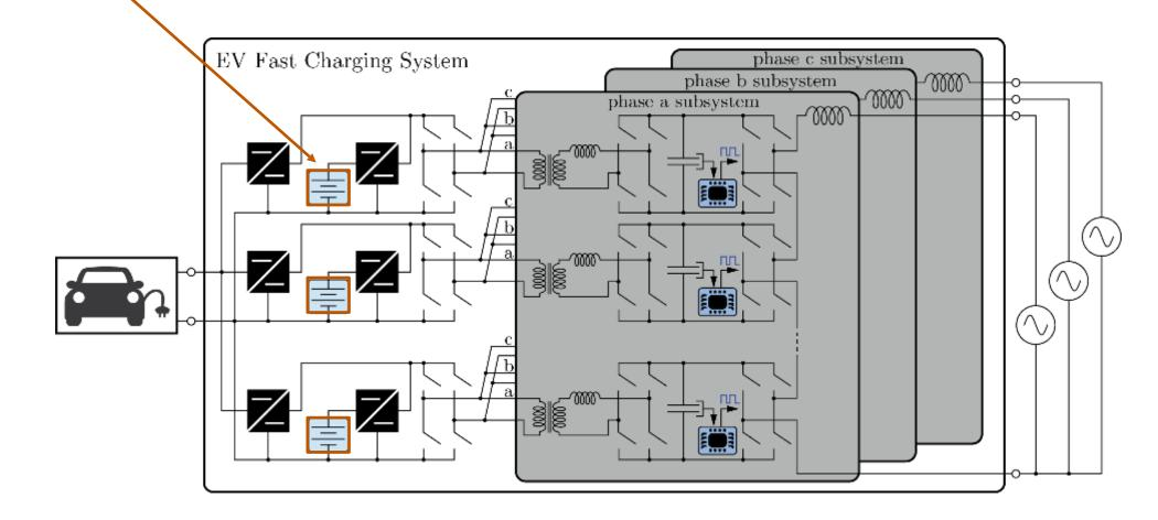
Dc and ac side controls work together and mimic power low pass filter from grid perspective
