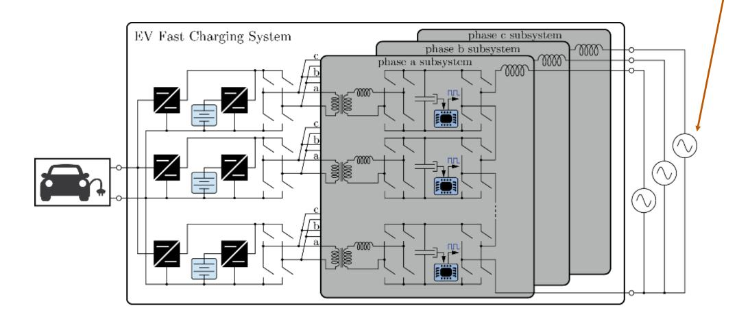
Distributed stationary storage to smooth out grid-side demand & reduce distribution capacity
