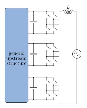
Upstream structure abstracted away & focus on one leg of H-bridges from here forward
