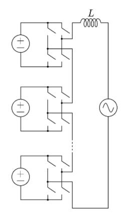
Upstream structure abstracted away & focus on one leg of H-bridges from here forward
