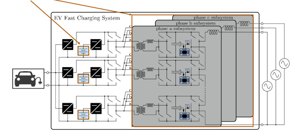
Distributed stationary storage to provide real/reactive power to support grid
