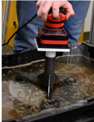
*Figure 17: Palm sander installation method being used to install foundation*
