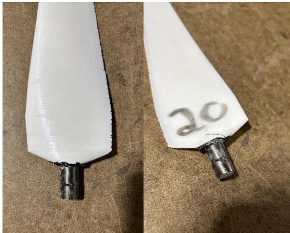
Figure 3: PLA blades with carbon fiber wrapped roots.
