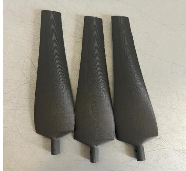
Figure 4: Carbon Fiber SG6043 Blades
