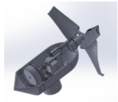
Figure 19. Section View of Nacelle Mechanical Design
