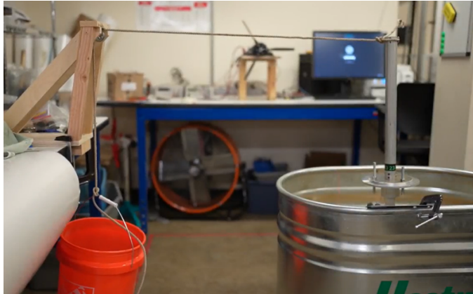
Figure 16. Experimental setup of the structural stability test. The foundation is mounted to competition testing specifications in the metal horse trough on the right side of the image.
