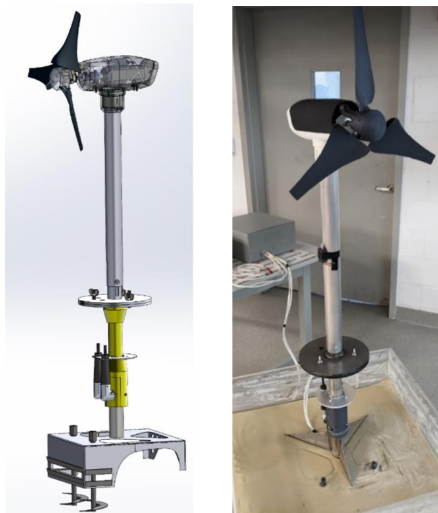
Figure 1: Turbine solidworks (left) Turbine Prototype (right)
