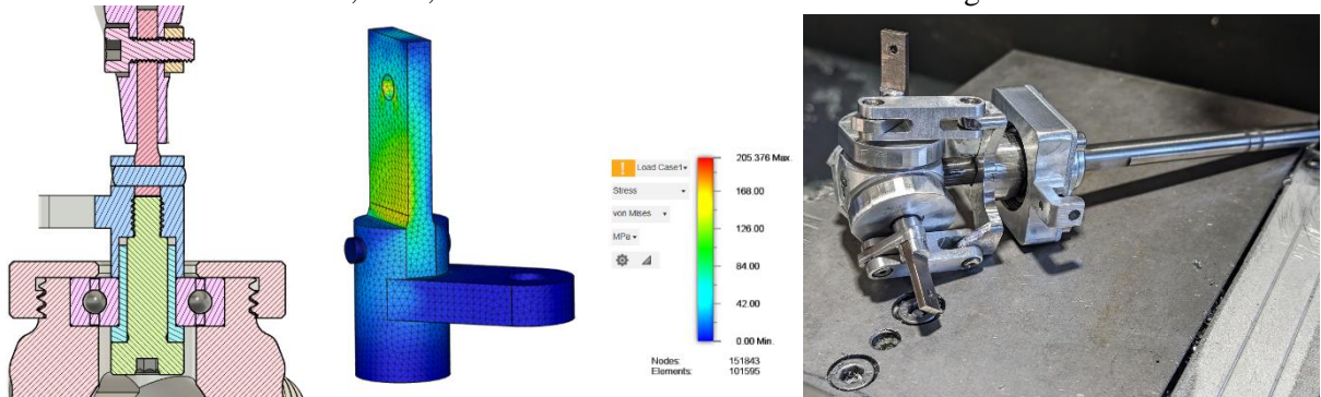
Figure 6. Section of blade spar stack, FEA study of loads in the spar, and photo of finished assembly.
