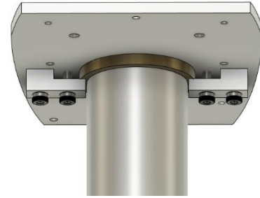
Figure 7. (Above) View of the yaw clamping lock on underside of nacelle plate.
