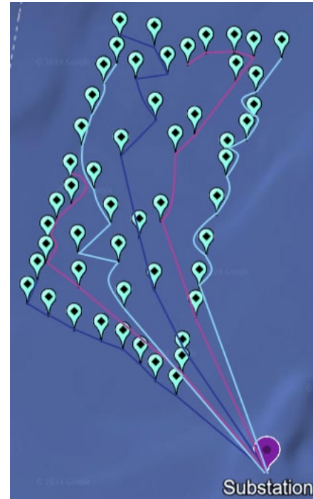
Fig 6. Turbine Layout Connections
