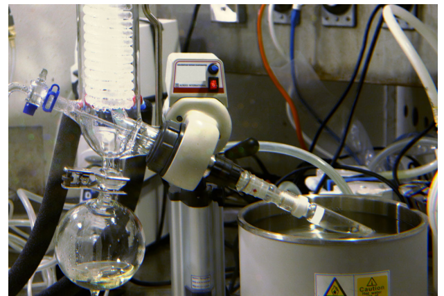
Extracting thorium-229 from U-233 prior to processing and disposal.
