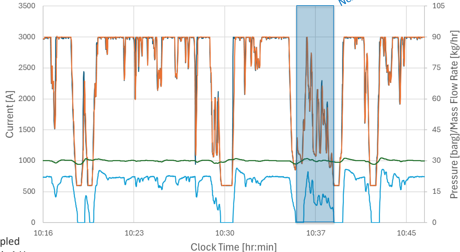
Electrolyzer Operation with 1.5 MW Wind Turbine Curve (Normalized to 1.25 MW)
