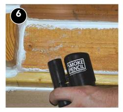
By sealing at the top of the cavity, airflow is stopped and no air movement should be visible when checking your work with smoke at a test pressure of 50 pascals.
