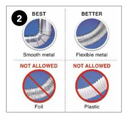
Duct material is rigid or semi rigid metal.
