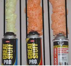
One-part spray foams can also span up to 3 inches to create an air seal.
