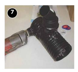
Use hand tools or shrouded power tools attached to a HEPA vacuum to limit the spread of dust and debris.
