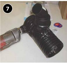
Utilize hand tools and/or shrouded tools attached to a HEPA vacuum that minimize dispersion of dust and debris.
