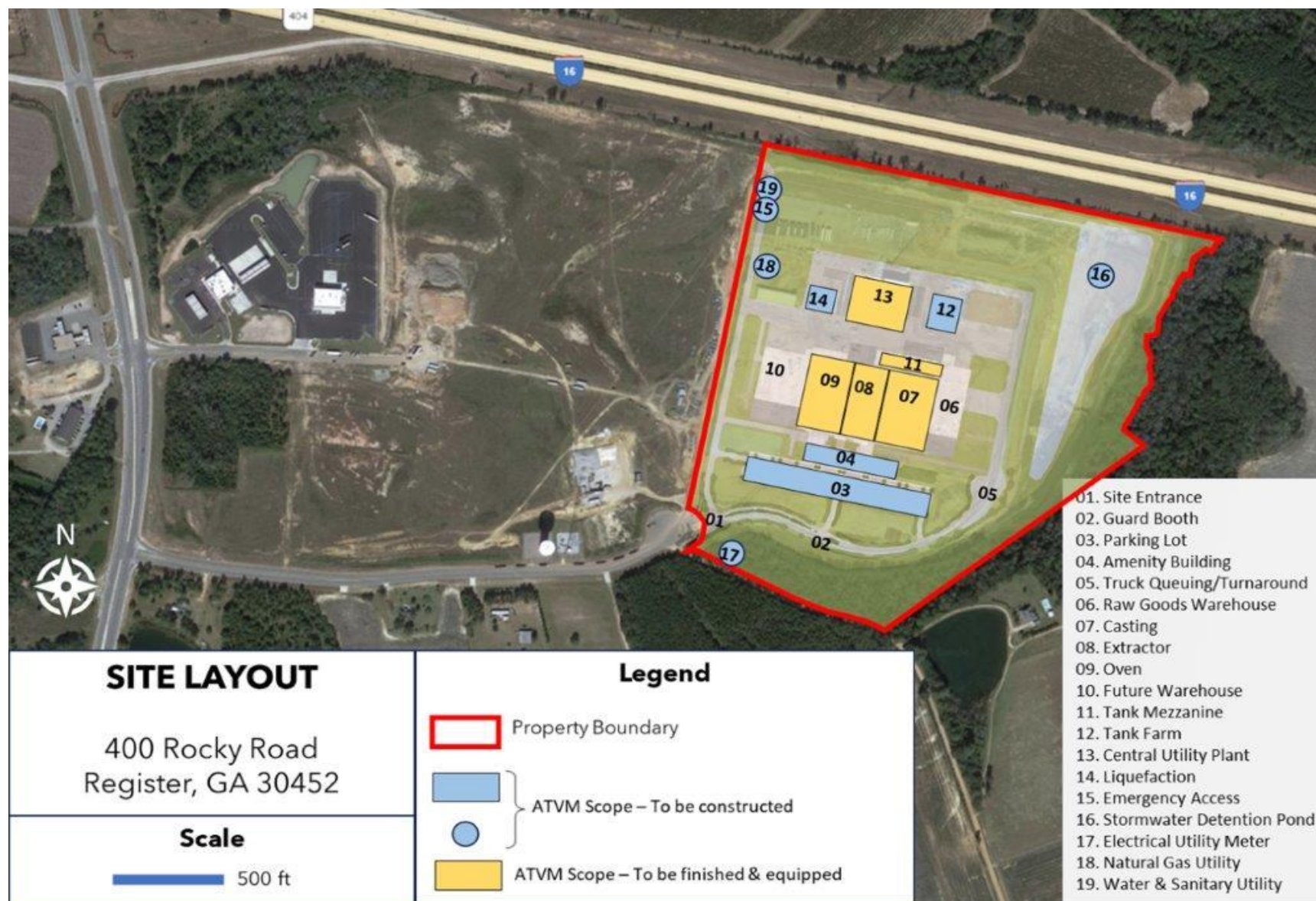
Figure 2-1: Detailed Site Layout
