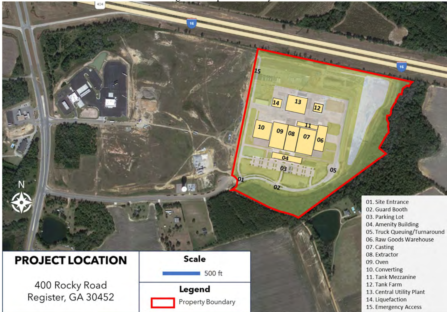
Figure 2. Proposed Site Layout
