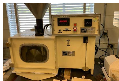
Figure 3. Laboratory-scale equipment to rapidly characterize MSW abrasiveness using a method based on an ASTM-approved test standard (G65)
