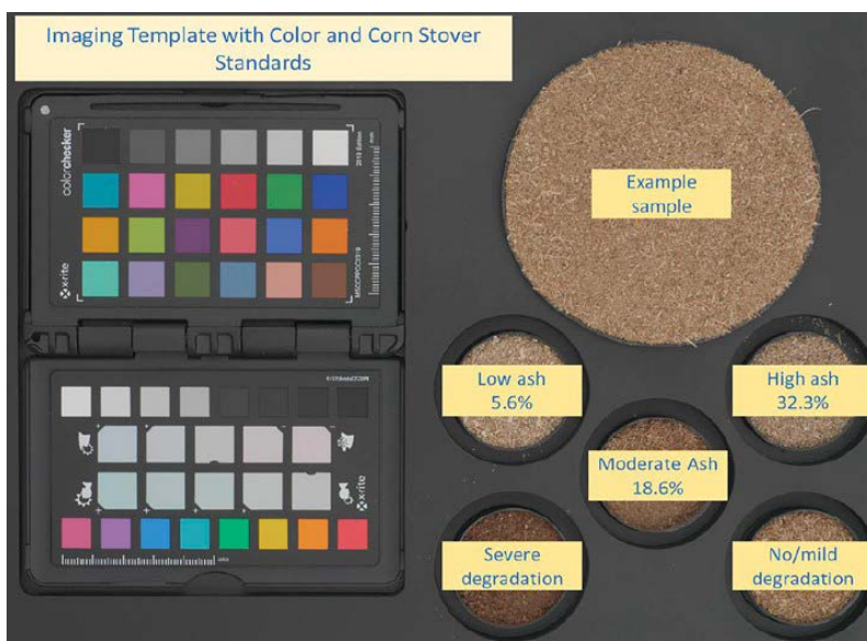
Figure 7. Image analysis tools can help screen and classify biological degradation and soil contamination in corn stover.
