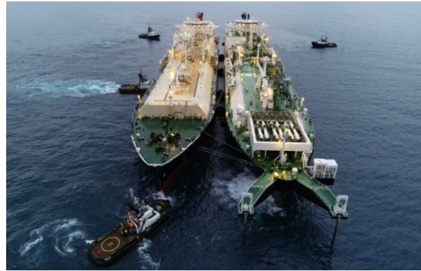
Figure 4 SSY mooring system on FSRU offshore Brazil
