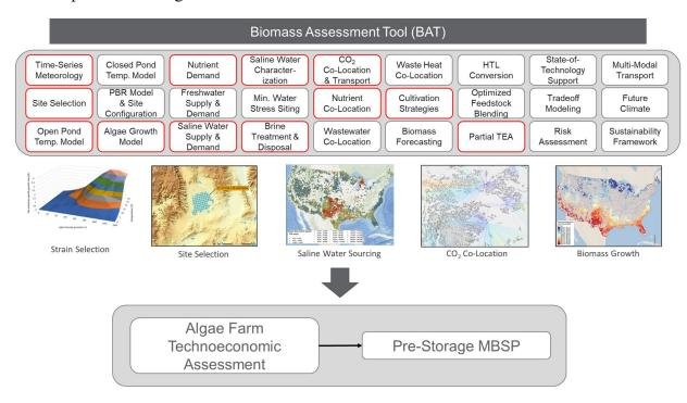
Figure 7.5. Components and workflow for microalgae resource analysis and TEA for BT23. The red highlighted boxes indicate the BAT modules used in this assessment.
