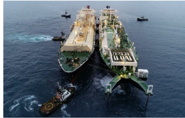
Figure 4 SSY mooring system on FSRU offshore Brazil
