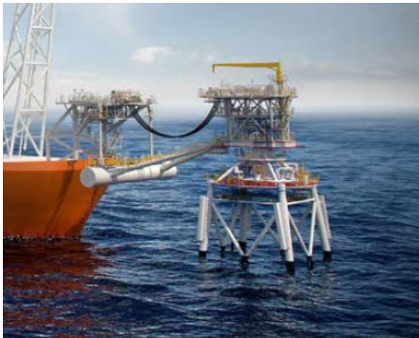
Figure 1 Tower Yoke Mooring System
