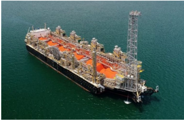
Figure 3 SSY mooring system on FLNG offshore Cameroon
