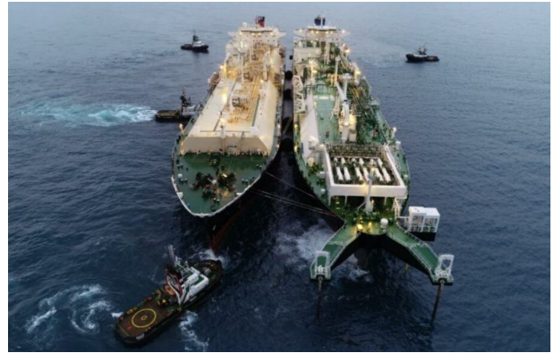
Figure 4 SSY mooring system on FSRU offshore Brazil
