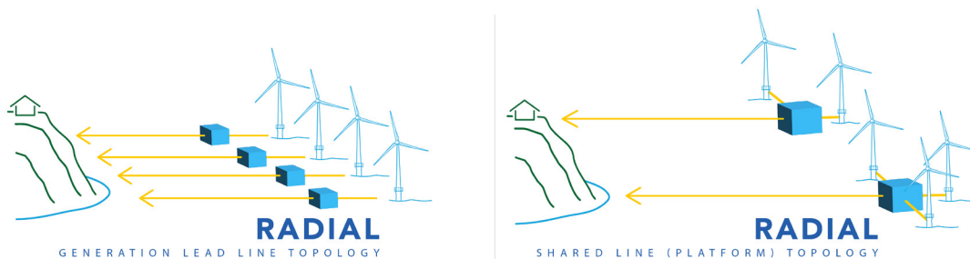
Figure 7. Radial transmission topologies (offshore wind plants represented as single turbines).
