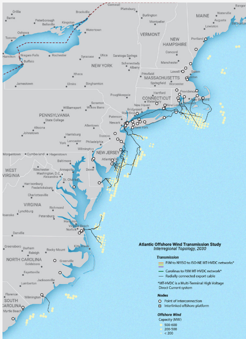
Figure 2. Map of potential offshore transmission development by 2030 for the Low Carbon Scenario, based on analysis of the AOSWTS.
