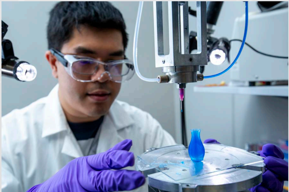
LLNL physicist Du Nguyen inspects a tiny flower vase printed using Tailored Glass by Direct Ink Writing technology, where the flow rate of two different glass-forming inks is adjusted to control the material composition emerging from the nozzle during the build. Photo credit: Jason Laurea
