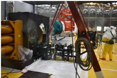
N3B Waste Retrieval Operations crew guide a cut section of corrugated metal pipe filled with cemented transuranic waste into a standard waste box in preparation for shipment and permanent disposal at WIPP.
