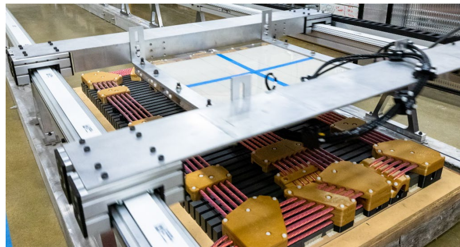
The dynamic inductive charging emulator used for the validation of 200-kW DWPT system in the laboratory
