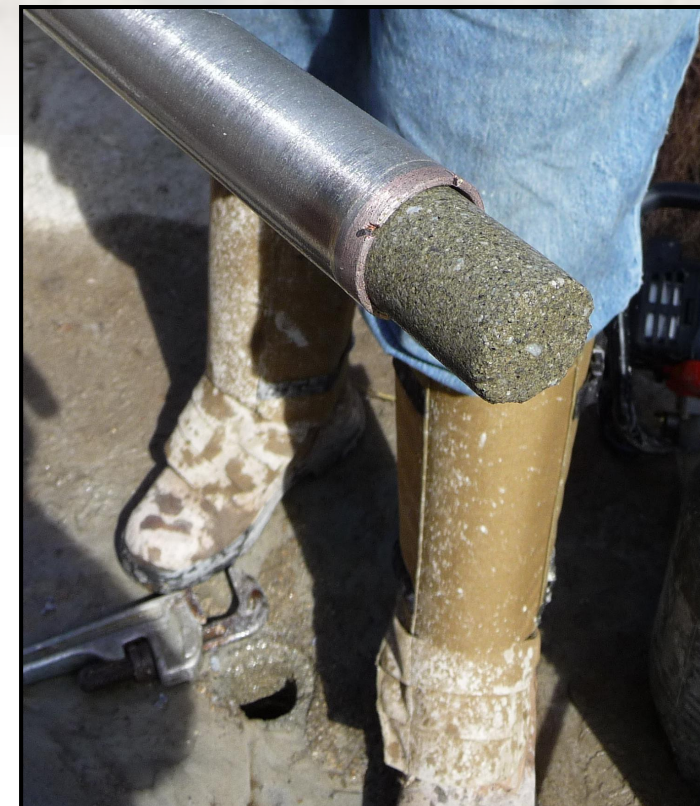
Field set-up for coring horizontal holes.
