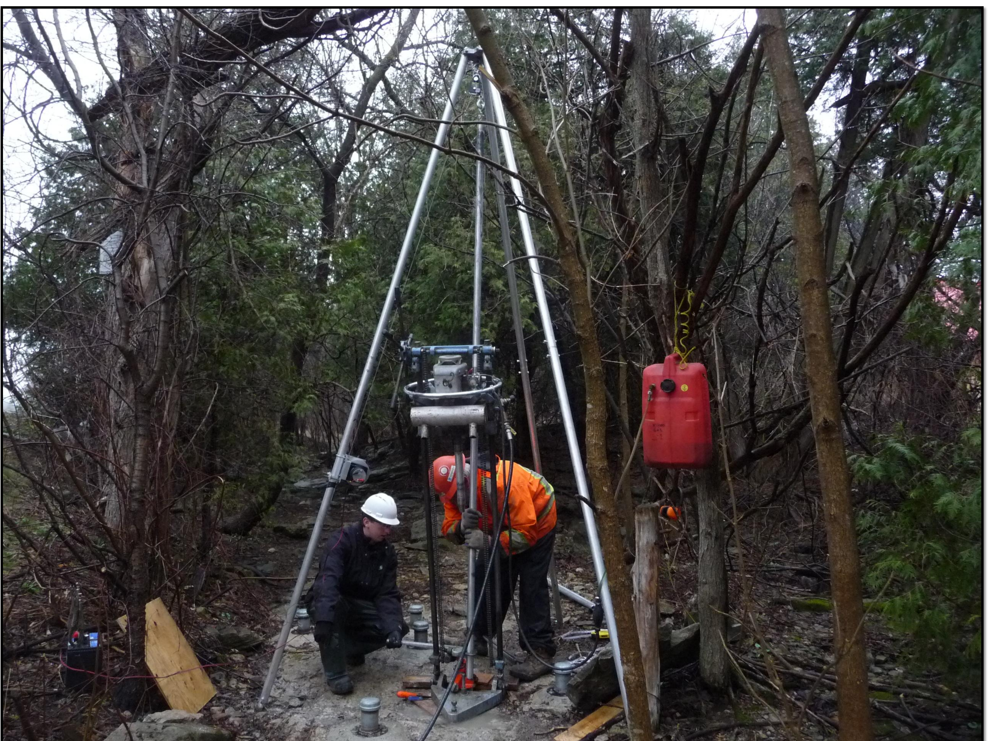
The Winkie Drill cores to depths > 50' with a 1.89" diamond drill bit.
