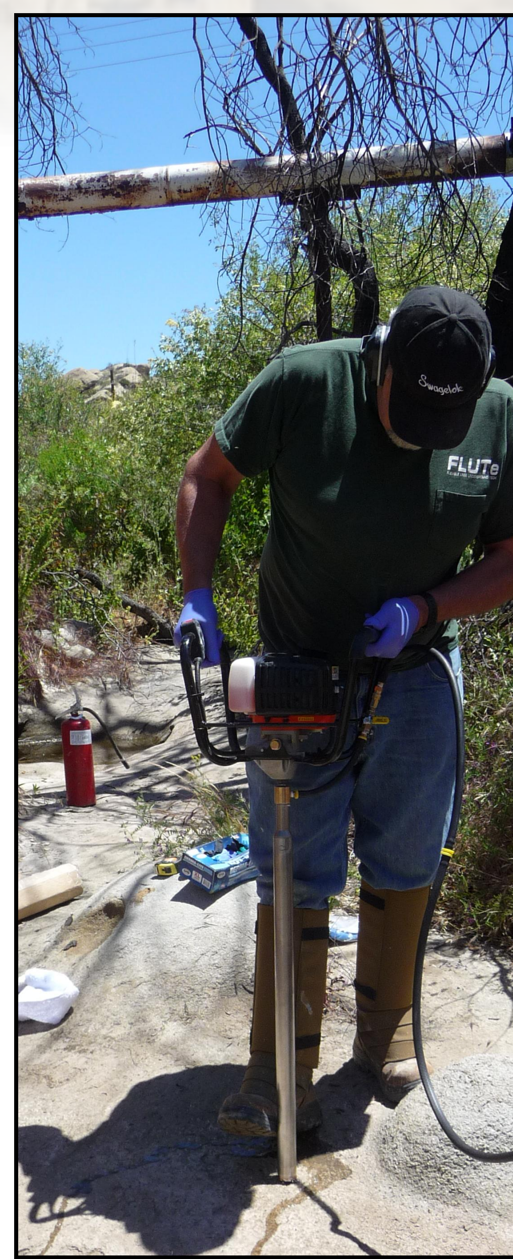
← Field set-up for coring vertical holes.
