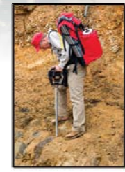
Shaw Back-Pack Core Drill Shallowest Drilling ~20 ft
