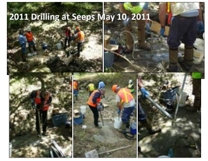
The Shaw Back-Pack Core Drill was used in May 2011 to core to a maximum depth of 20 feet.
