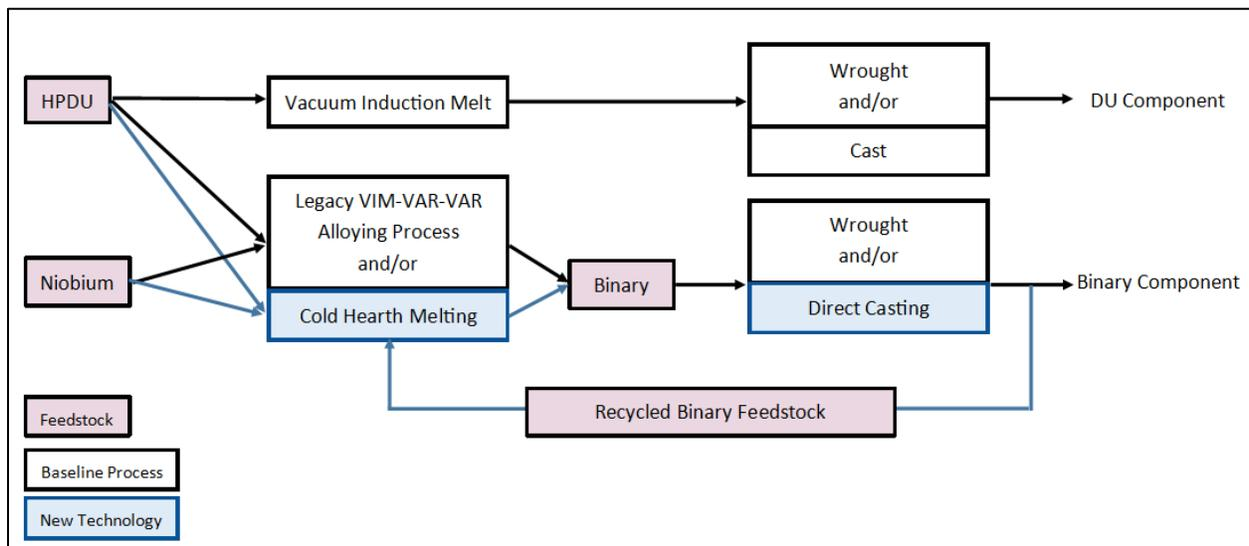
**Figure 3–1. Potential production process with new technology insertion**
