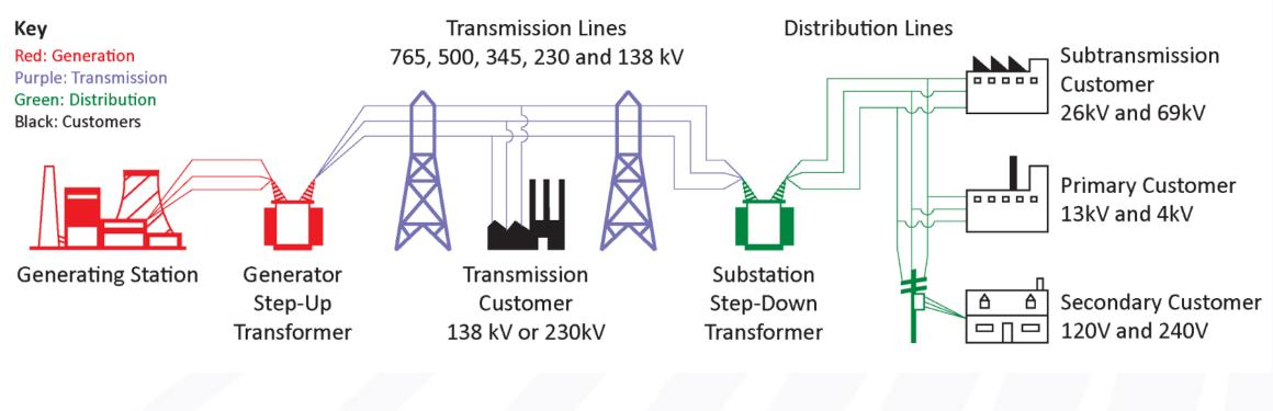
Note: 161 and 115 kV Transmission Voltages Exist Note: 46, 34.5, 23 kV and other Distribution Voltages Exist
