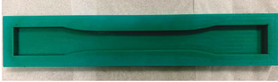
Figure I.1.14.1 Silicone mold for the fabrication of dog bone test structures.
