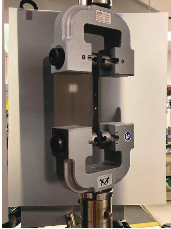
Figure I.1.14.4 Picture of a Fe 4 N/epoxy composite undergoing tensile testing at NREL.
