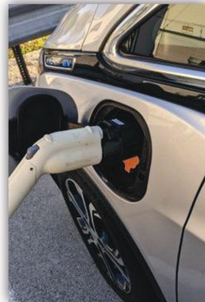
Figure II.4.1.7 Smart Charge Adapter with OCPP 1.6J client charging Chevrolet Bolt.
