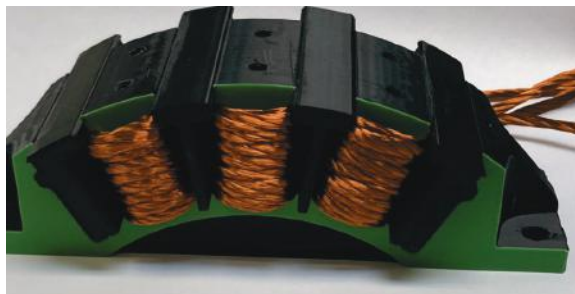
Figure I.1.3.2 Winding trials on a 3D-printed stator core.
