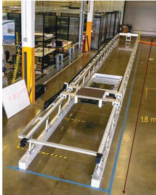
Figure II.3.1.4 Top view of the ORNL DICE depicting the overall track length of 18 m.
