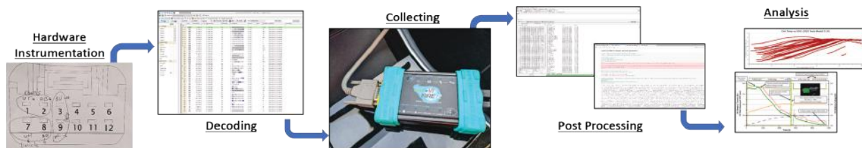
Figure II.2.1.2 Process for vehicle data collection used throughout process
