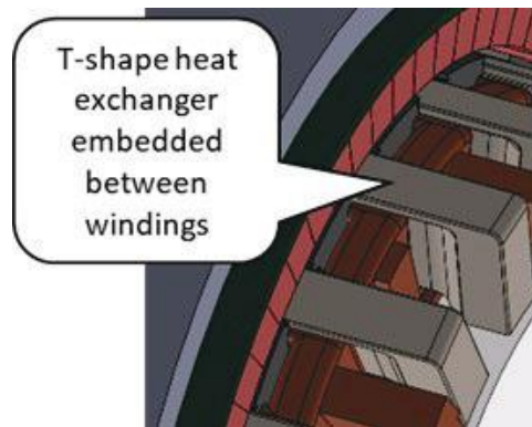
Figure I.1.7.4. T-shape heat exchangers embedded between stator windings. Illustration by Bidzina Kekelia, NREL
