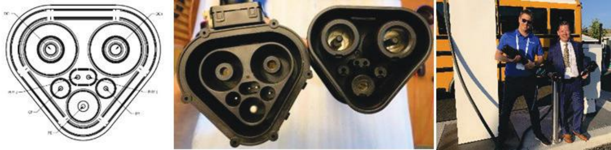
Figure II.6.2.3. SAE J3271 MCS coupler; pin functions, pre-production examples, Portland OR demonstration
