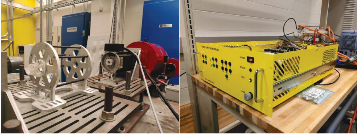
Figure I.1.19.7 Prototype DHAM frame (left) and inverter (right).
