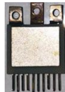
Figure I.1.24.4 A fabricated double-side cooled SiC phase-leg power module encapsulated by EP-2000 for 200°C-T j operation.
