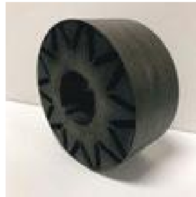
Figure I.1.16.4 Fabricated HF-10 rotor lamination
