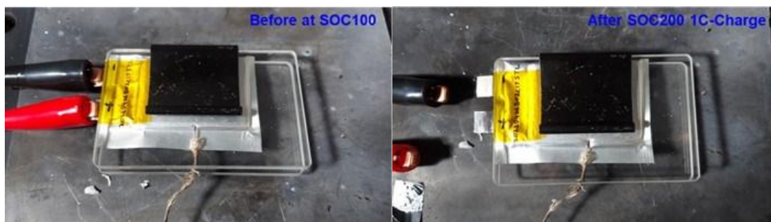
Figure I.3.49 Slight gassing observed after the 200% SOC overcharge.
