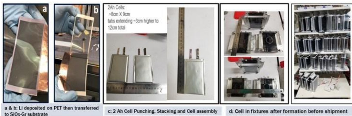
Figure I.7.1 (a & b) Examples of silicon (SiOx) anode showing transfer of Li to anode. (c) Cell sizes and dimension for final BP-1 deliverable, and (d) Pouch cell assembly process - Cells in fixtures going through formation and cycling before shipment
