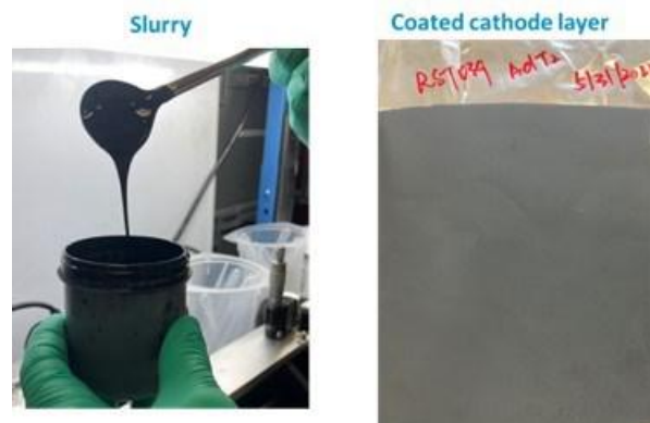
Figure XI.1.12 SAFT experiments: slurry and cathode layer made with alumina surface coated RST 9055
