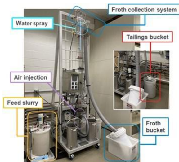
Figure III.3.9 Froth flotation column set-up at Argonne National Laboratory
