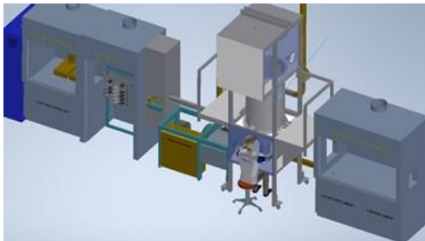
Figure II.2.4 FSP configuration for 500 g/hour production
