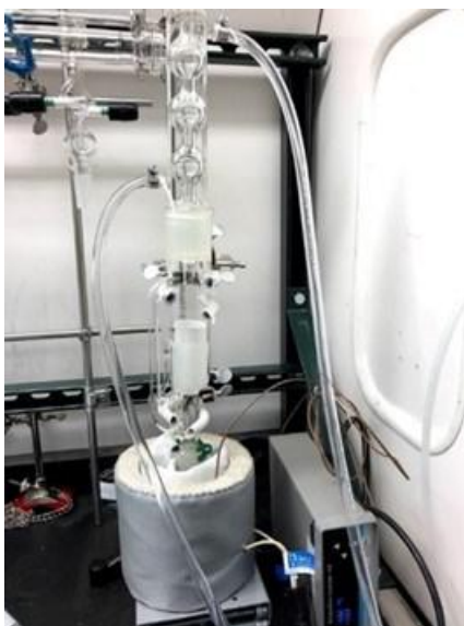
Figure III.3.5 Conventional Soxhlet extractor design
