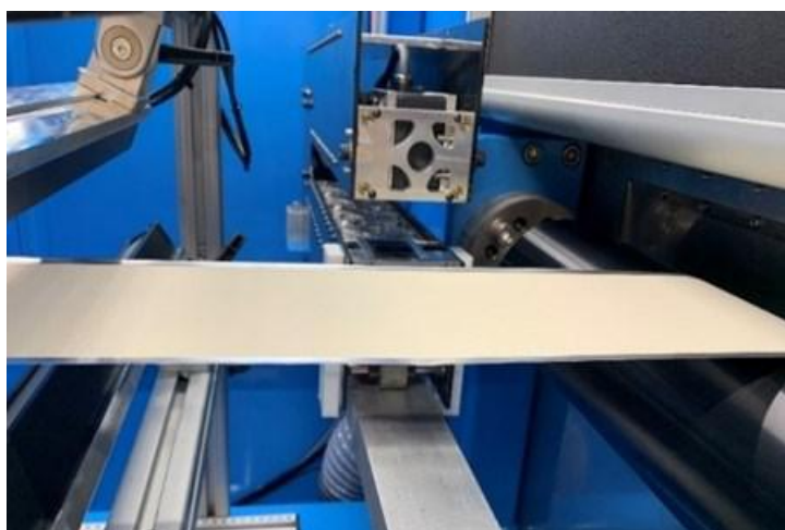
Figure XVI.2.2 A solid-state-electrolyte separator coating on a slot-die coater
