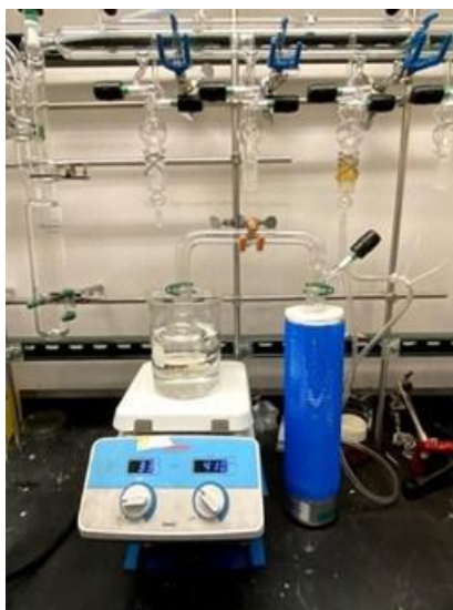
Figure III.3.6 PVDF binder and cryovap solvent transfer apparatus
