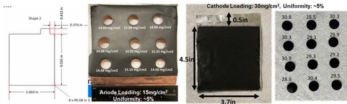
Figure I.5.6 5Ah cell electrode preparation for testing at WPI and Microvast.
